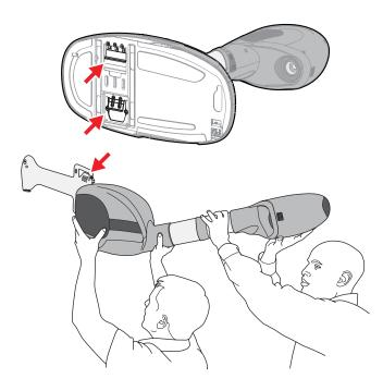
9. Using 2 people, slightly push up on the unit to make sure unit is locked on mounting plate
